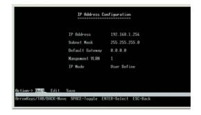
Figure 4-15: IP Address Configuration
